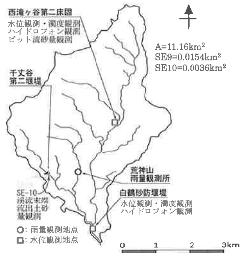
図-8 住吉川における流砂量等観測位置 Fig.8 Sediment discharge observation positions in the Sumiyoshi river
