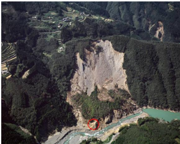
Fig. 2. Nonoo landslide dam after collapse.
