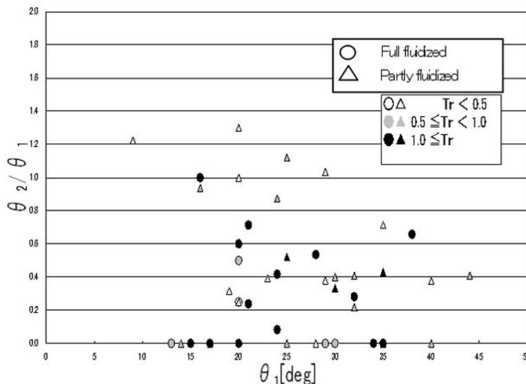
Fig. 8. Inclination of landslide and the lower side in end of landslide and traveling ratio.
