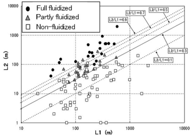
Fig. 11. Relationship between the length of landslide (L1) and travel distance (L2).
