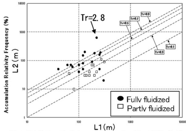
Fig. 15. Relationship between the length of landslide (L1) and travel distance (L2). (Landslides generated by Chuetsu earthquake)
