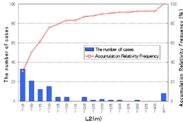
Fig. 2. Histogram of the travel distance of landslides.
