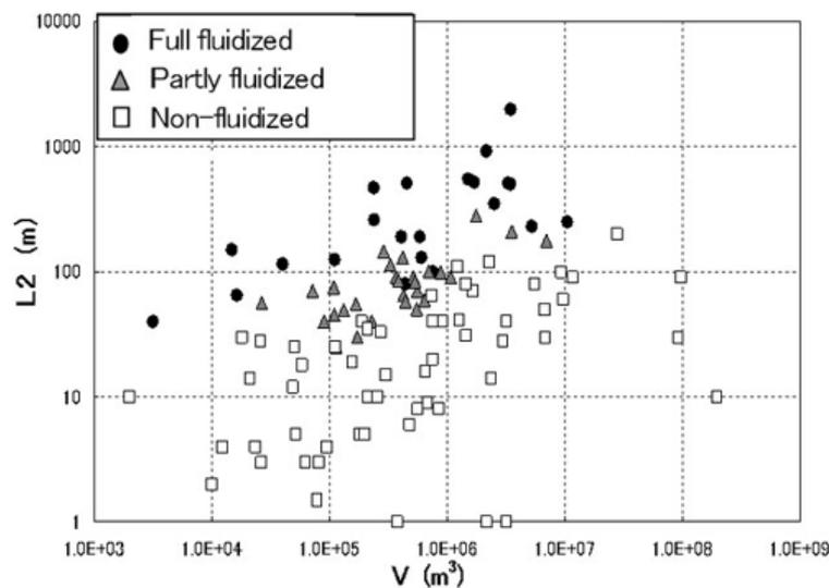
Fig. 10. Relationship between landslide volume ( $V$ ) and travel distance ( $L_2$ ).
