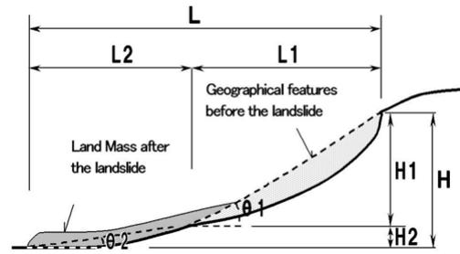
Fig. 1. Definition of factors on landslide movement.
