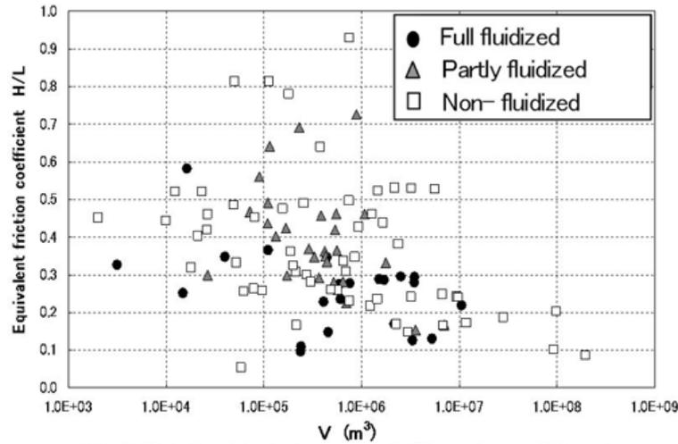
Fig. 9. Relationship between landslide volume ( $V$ ) and the equivalent friction coefficient ( $H/L$ )
