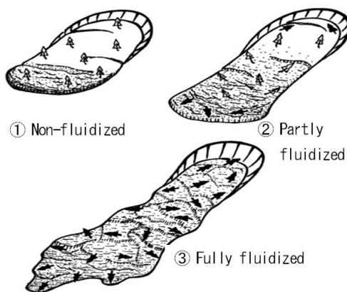
Fig. 7. Classification of landslides from their movement.
