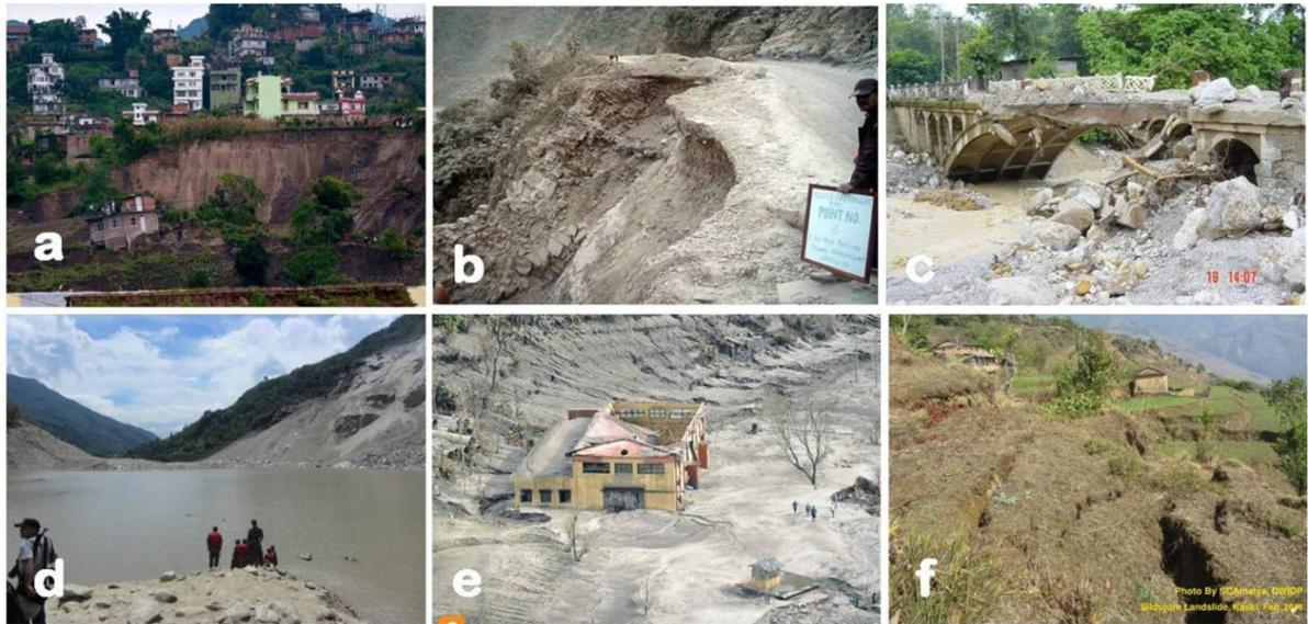
Figure 3. Landslide disaster affecting to a) Settlement: Tinthanalandslide, Kathmandu, b) Highway: Mugling-Narayanghat highway, c) Bridge: Mugling-Narayanghat, d) River damming: Sunkoshi River, Jure landslide, e) Hydropower: Sanima hydropower, Jure landslide, f) Agricultural land: Sildujure landslide Kaski (source: DWIDM).
