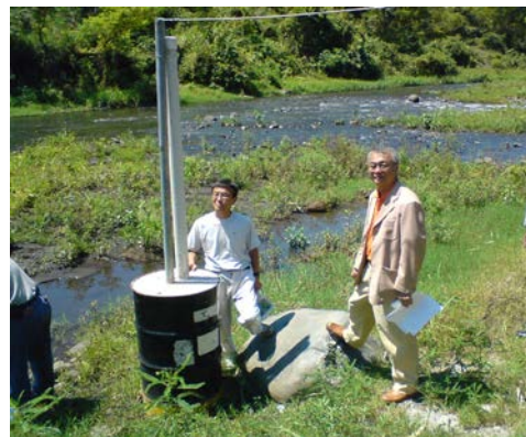
Photo 7 Water level gauge on the concrete Basement (Guatemala)
