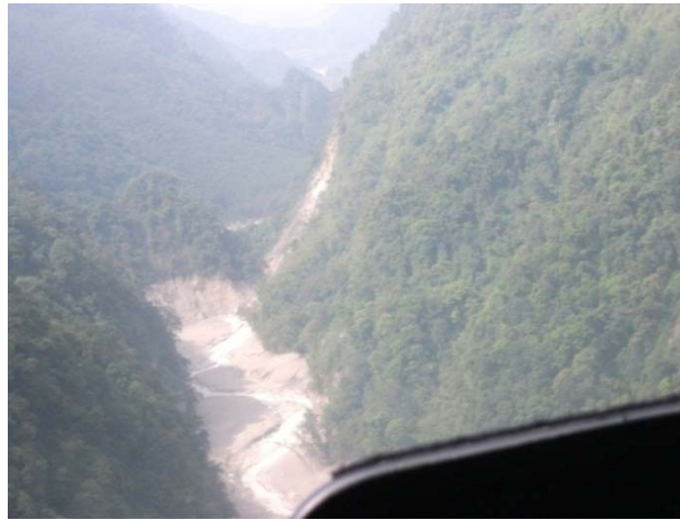
Image 6.4.2 River bank erosion and slope failure at the narrow bend of the Seti River
